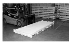
To take on pallets from their long side, position the forks at a distance of at To take on pallets from their short side (e.g. when unloading containers), least 1 meter (39") from the other, perpendicular to the long side of the pallet you must use forks with a length of at least 84" to guarantee a sufficient and at the center. Forks must be supporting the entire surface of the pallet.
