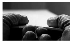
After scoring, it is sufficient to bend the slab to detach the two pieces.
