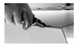
As far as THINNER 3plus and THINNER 5plus are concerned, after scoring and splitting the slab, complete the operation by cutting the fiberglass mesh with a razor knife.
